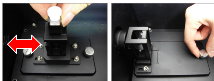
Fig. 6. Comparison between the Fluorescence Microcell Holder (Left) and the Luminescence Microcell Holder (Right)
